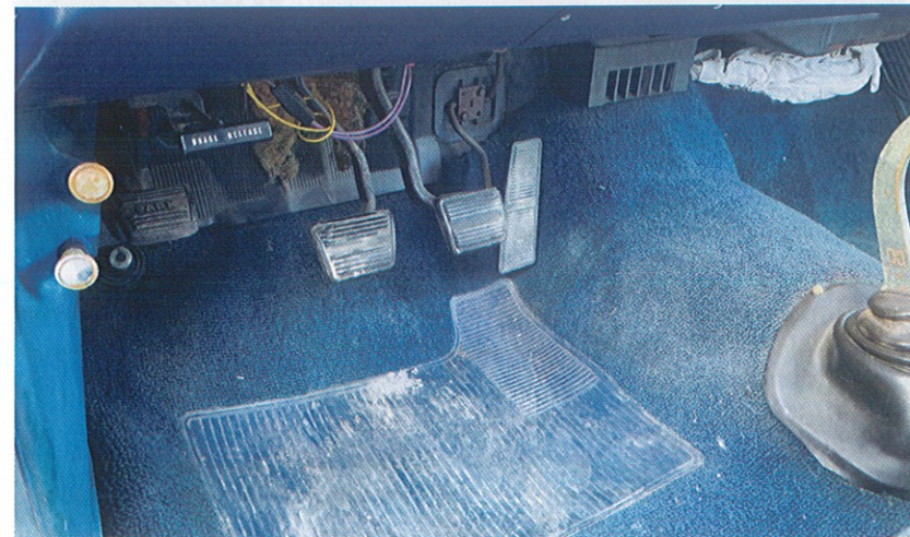
That's the original carpet and Hurst 4-speed shifter. Check out the towel stuffed under the heater. We don't know how long it's been there but failed heater cores are common when an old muscle car sits for long periods.
